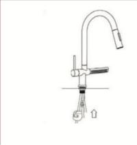
Screw and tighten the flexible hoses to the faucet. Do not allow the water supply brass tube to twist.
