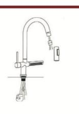
After installing faucet remove spray assembly and open the hot and cold water supplier. Check for leaks. Turn on faucet handle for one minute to flush debris from faucet. Turn off the handles and re-assemble the spray.
