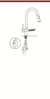
Proper installation of the hose weight kit ensure it can pull smoothly. Measure 15" from the bottom of the faucet. Faucet mount hose weight kit at this point, I'm going to put a label here. Easy to move and smooth to retract. Repositioning hose necessary weight kit. Ensure that the hot and cold supply hoses do not interfere with the hoses. Adjust the position slightly if necessary.
